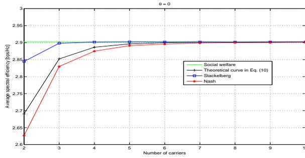
Fig. 10. Average spectral efficiency with independent users.
