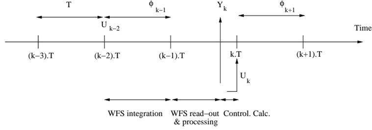
Fig. 2. Temporal diagram of the system process.
