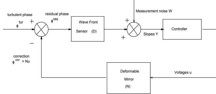
Fig. 1. Block diagram of a classical AO system closed-loop.
