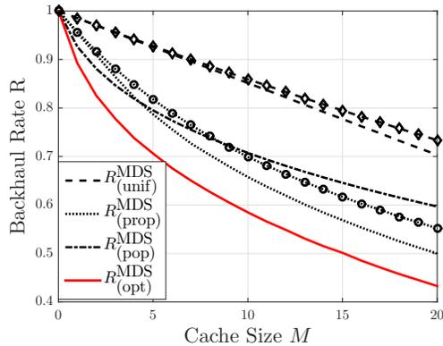
Fig. 4. Backhaul rate as a function of the cache size  $M$ , with  $N=200$  files,  $\alpha = 0.7$  and  $r = 60$  meters. The lines without markers depict the use of MDS codes (encoded packets) in the placement, while the line with markers depict uncoded (fragments) placement.
