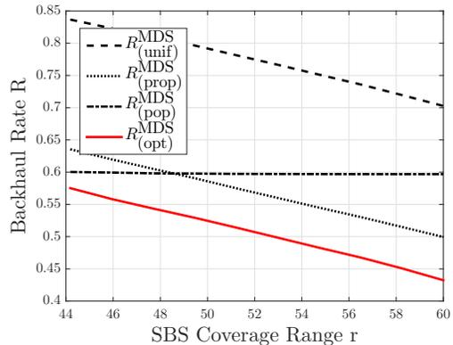
Fig. 5. Backhaul rate as a function of the SBS coverage radius  $r$ , with  $N = 200$  files,  $\alpha = 0.7$ , and  $M = 20$  files.
