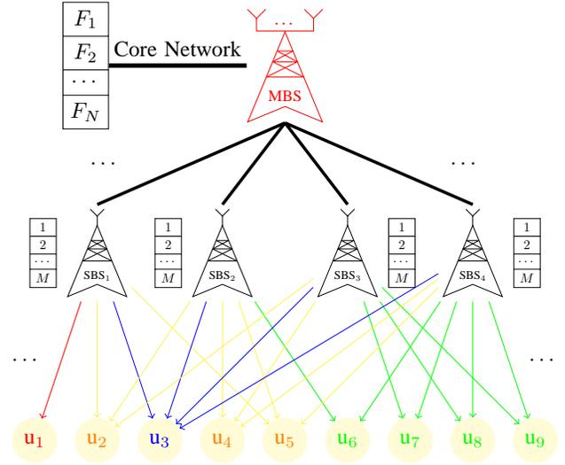
Fig. 2. Instantaneous Heterogeneous network topology.
