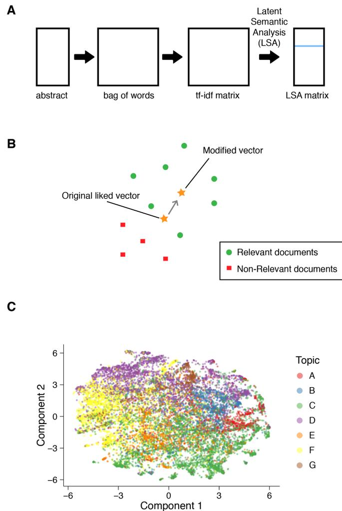
**Fig 1. Vector representation of documents** (A) Schematic of the workflow for converting abstracts into vector representations (see Algorithm 1) (B) Schematic of Rocchio Algorithm (C) Projection of SfN abstract vectors to 2-dimensional space using *t*-SNE color coded by human curated sessions from A to G
