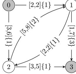
Figure 1: Example of an R-RSP instance, with origin  $o = 0$  and destination  $t = 3$ . The notation  $[l_{ij}, u_{ij}]\{d_{ij}\}$  means, respectively, the cost interval  $[l_{ij}, u_{ij}]$  and the resource consumption  $\{d_{ij}\}$  associated with each arc  $(i, j) \in A$ .
