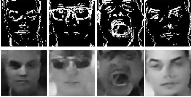
Figure 10: Intensity reconstruction result inferred by the network described in Section 5 and trained on the WIDER simulated data. The top row shows 64x64 face crops captured with the prototype camera, the bottom the corresponding reconstructed images. While the quality is not quite on par with the intensity reconstructions, it has to be noted that the resolution of the crops in Figure 8, is 96x96, *i.e.* 1.5x larger.
