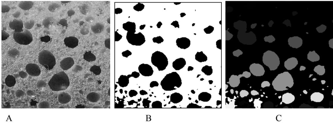
**Figure 9:** A is the grey-tone image (240 x 240 pixels). B is the image after thresholding and C is the result of segmentation. As in the previous cases, we have some super-pixels which are so dark that are not visible in the map.
