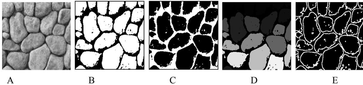
**Figure 3:** A is the grey-tone image (240 x 240 pixels). B is the image after thresholding. C is B inverted (the inversion of tones is necessary since the program works on black pixels). D is the result of segmentation. The super-pixels are given in grey-tones. Since some of these super-pixels are dark; they are shown by an edge detection, as given in the E panel.
