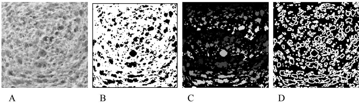
**Figure 10:** A is the grey-tone image (240 x 240 pixels). B is the image after thresholding and C is the result of segmentation. D is the result of edge-detection.
