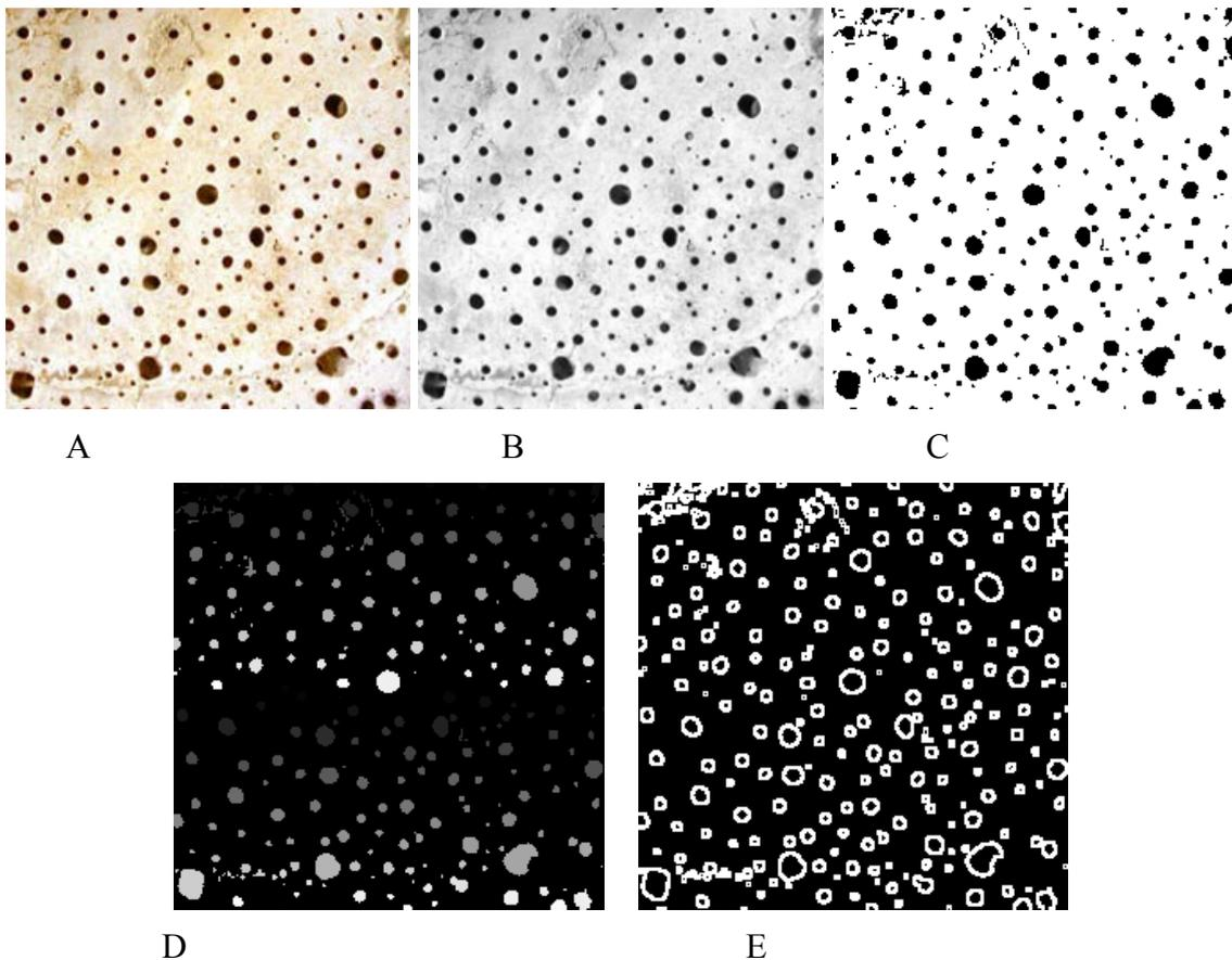
**Figure 5:** A is the original image (240 x 240 pixels). B is its grey-tone image. C is after a thresholding. D is the result of segmentation according to the Fortran program discussed above.
