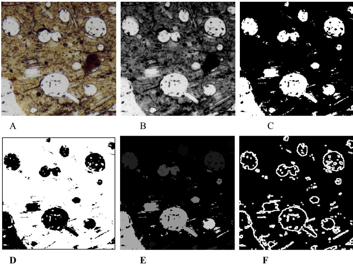
**Figure 8:** A is the original image (240 x 240 pixels). B is the corresponding image in grey tones. C is after thresholding. D is the same as C, but with black and white tones inverted. E is the result of segmentation, and F the image after edge-detection.
