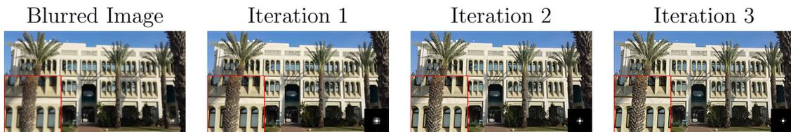
Figure 8: PROBE deblurs an out-of-focus image obtained with a smartphone. Displayed: The blurred image and PROBE results by iteration with the corresponding shrinking residual blur kernels superimposed.
