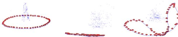
Figure 1: In many structure from motion pipelines, camera orientations are estimated with rotation averaging followed by recovery of camera centres (red) and 3D structure (blue). Here are three solutions corresponding to different local minima of the same rotation averaging problem.
