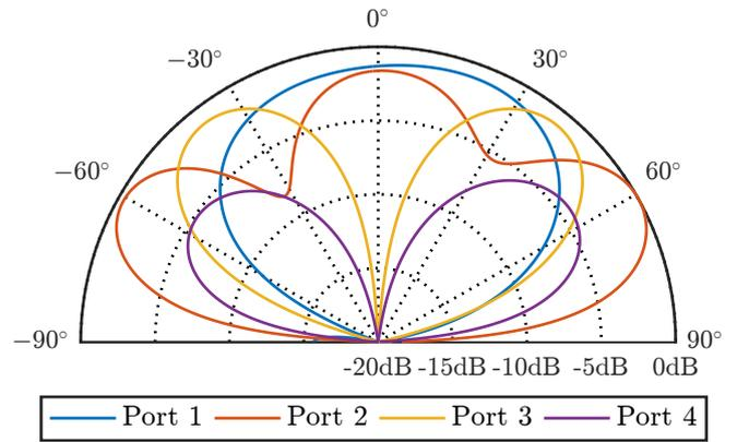
Fig. 2. MMA  $x$ - $z$  plane power patterns for RHCP
