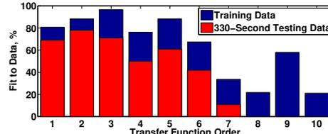
Fig. 6. The figure shows how optimal transfer functions with different orders and zero relative degree fit the  $y$ -direction training and testing data. The NRMSE fitness measure is used. The dynamic order 3, proposed by our algorithm, best fits the training data, and it achieves the second highest fit to the 330-second testing data.
