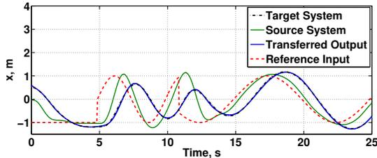
Fig. 4. The training input-output data used to identify the transfer learning map in the  $x$ -direction, and the transferred output using the proposed map. The transferred output fits the target system's output with 95.79%.
