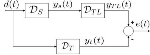
Fig. 2. Illustrative figure of the transfer learning problem: the objective is to identify a transfer learning map  $\mathcal{D}_{TL}$  to minimize the error between the transferred output  $y_{TL}$  and the target system's output  $y_t$ .
