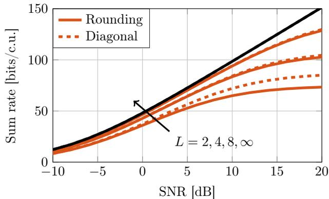
Fig. 6. Sum-rate with ZF and Gaussian signaling;  $B = 128$  and  $U = 16$ . The solid lines correspond to the rounding approximation in Section IV-B, the dashed lines correspond to the diagonal approximation in Section IV-C. The black lines, which overlap, correspond to the sum rate achievable in the infinite-resolution case.
