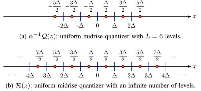
Fig. 2. Comparison between the quantization levels and thresholds associated with the rules  $\alpha^{-1}\mathcal{Q}(z)$  and  $\mathcal{R}(z)$ ; the red circles correspond to quantization labels, and the blue vertical lines correspond to the quantization thresholds.
