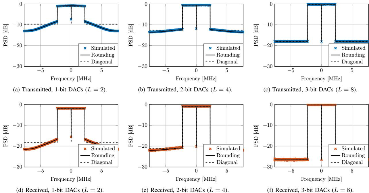
Fig. 3. PSD of the transmitted and received signal;  $B = 128$  and  $U = 16$ . The markers correspond to simulated values, the solid lines correspond to the rounding approximation presented in Section IV-B and the dashed lines correspond to the diagonal approximation presented in Section IV-C.
