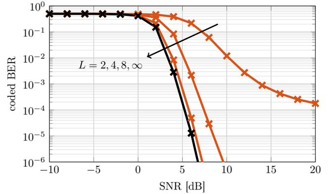
(b) Coded BER with 16-QAM;  $B = 128$  and  $U = 16$ .
