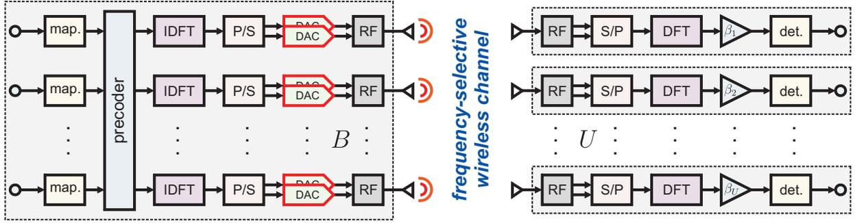
Fig. 1. Overview of the massive MU-MIMO-OFDM downlink with low-resolution DACs at the BS. Left: A  $B$  antenna BS performs linear precoding and generates the per-antenna OFDM time-domain signals that are passed through low-resolution DACs (highlighted with red color). Right:  $U$  single-antenna UEs perform independently OFDM demodulation and data detection. In the figure, “map.” and “det.” stand for mapper and detector, respectively.
