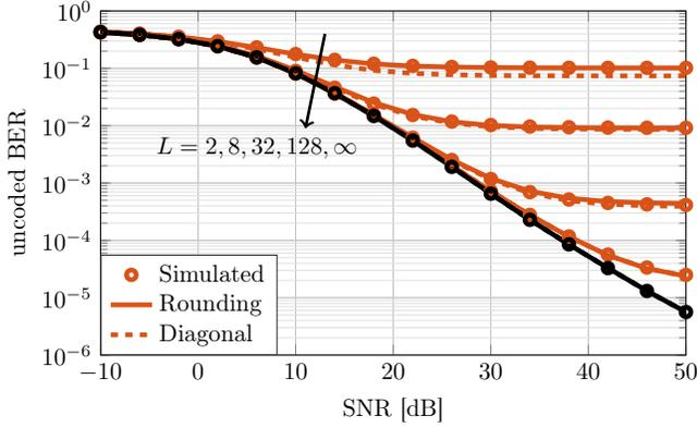
(a) Uncoded BER with QPSK;  $B = 1$  and  $U = 1$ .
