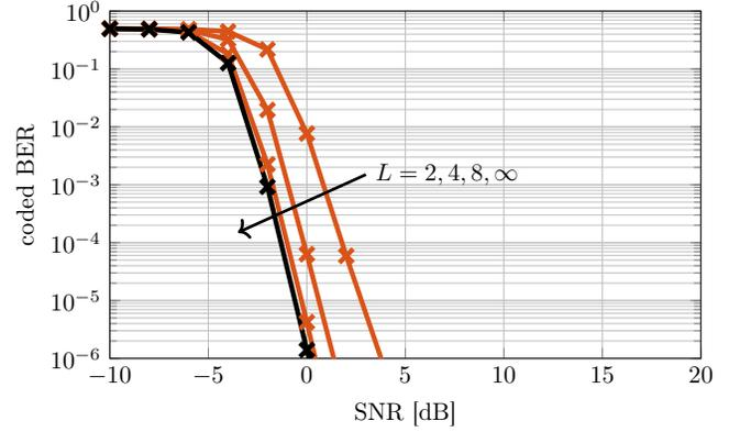
(a) Coded BER with QPSK;  $B = 128$  and  $U = 16$ .
