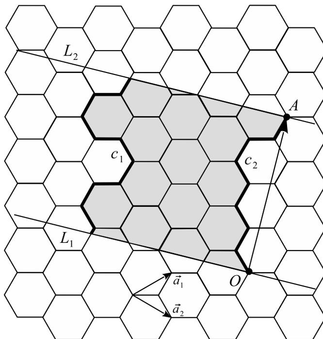
**Figure 2.** A tubulene of type  $(4, -3)$  with two basic lattice vectors.
