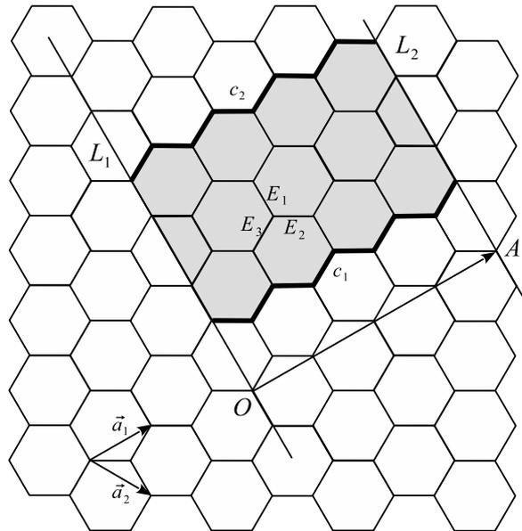
**Figure 4.** Zig-zag tubulene  $ZT(3, 4)$  with three directions of edges ( $E_1$ ,  $E_2$ , and  $E_3$ ).
