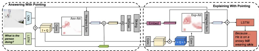
Figure 3: Our Pointing and Justification (PJ-X) architecture generates a multi-modal explanation which includes a textual justification (“He is on a snowy hill wearing skis”) and points to the visual evidence. Our model consists of two “pointing” mechanisms: answering with pointing (left) and explaining with pointing (right).
