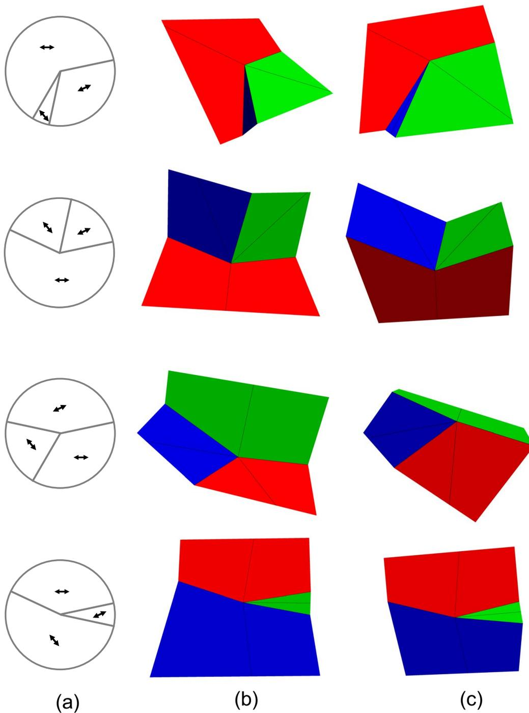
Figure 12: (a) Director design for the building block. (b),(c) The bi-stable actuations for  $r = 0.5$ .
