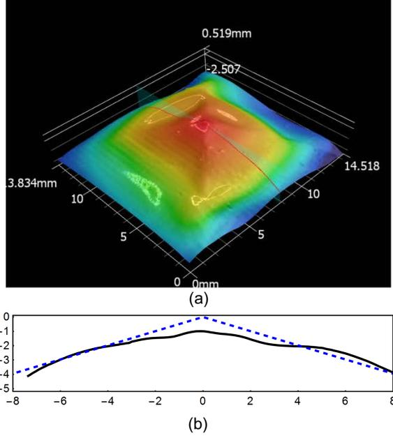
Figure 5: Experimental observation of the bias pyramid. (a) The actuated shape (the colors indicate elevation). (b) A comparison of the observed cross-sectional slice (solid curve) with the predicted cross-section for the unbiased design (dashed blue line).
