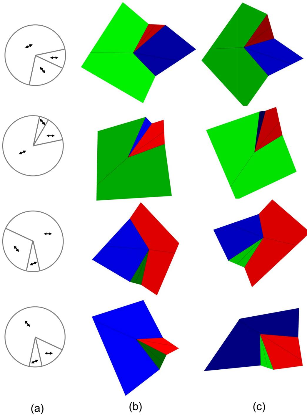
Figure 10: (a) Director design for the building block. (b),(c) The bi-stable actuations for  $r = 0.5$ .
