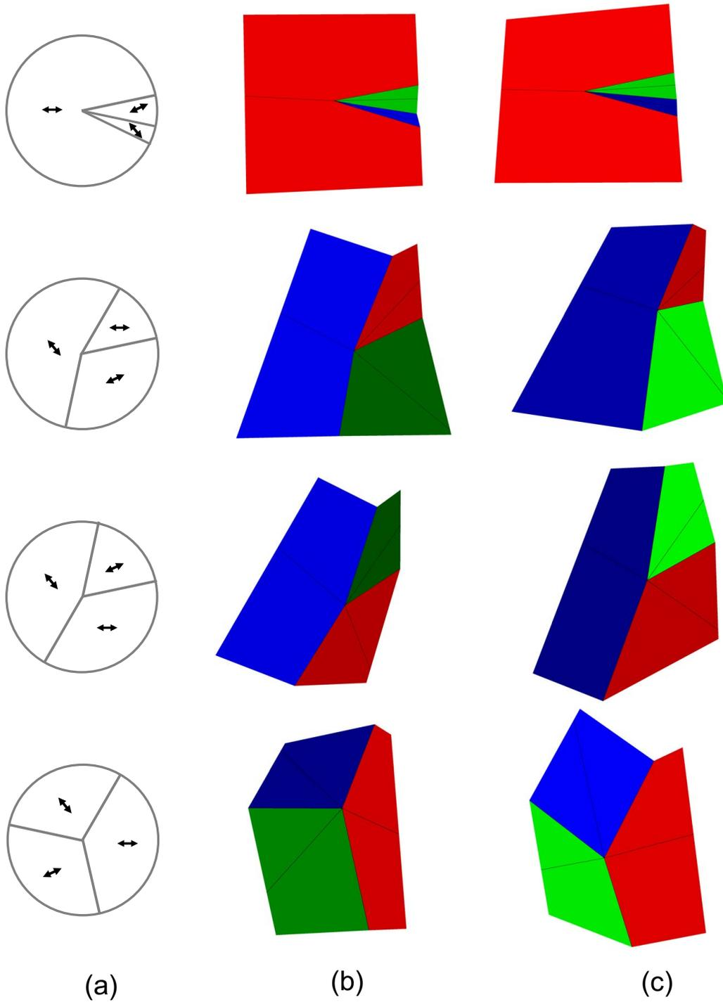
Figure 11: (a) Director design for the building block. (b),(c) The bi-stable actuations for  $r = 0.5$ .
