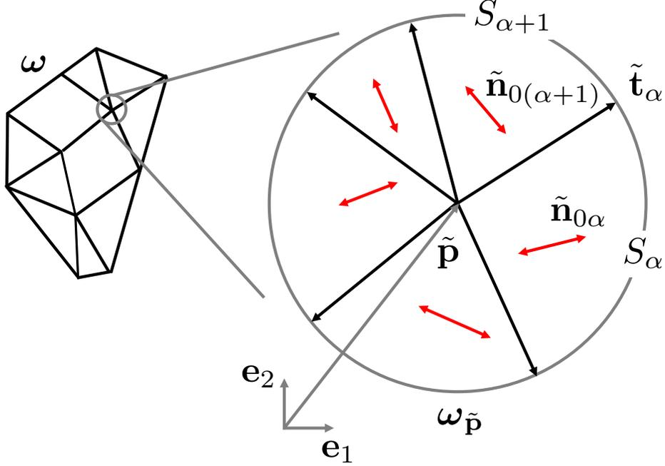
Figure 8: At each vertex, the actuation induced shape change of the sectors surrounding the vertex must be compatible for the pattern to be nonisometric origami.
