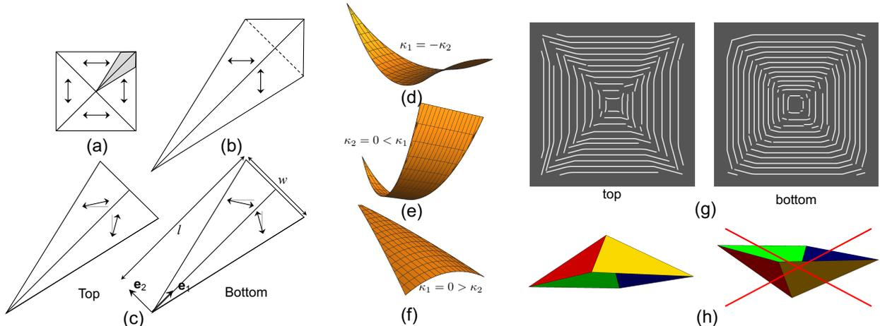
Figure 4: The design of a pyramid with bias. (a) The director pattern of non-isotropic origami pyramid and wedge-shaped region around an edge. (b) Details of the wedge-shaped domain highlighted in (a). (c) The modification of the origami director pattern to introduce a twist. (d-f) The possible actuated shape on heating of the triangular specimen shown in (c). (g) The director pattern for a biased pyramid. (h) The up pyramid is preferred over the down pyramid.
