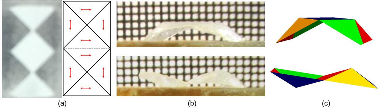
Figure 2: (a) The design and experimental realization for two linked symmetric four-faced building blocks (right and left respectively). (b) The sheet actuates into either of two degenerate and mechanically bi-stable configurations. (c) These configurations are predicted by theory, as discussed below.
