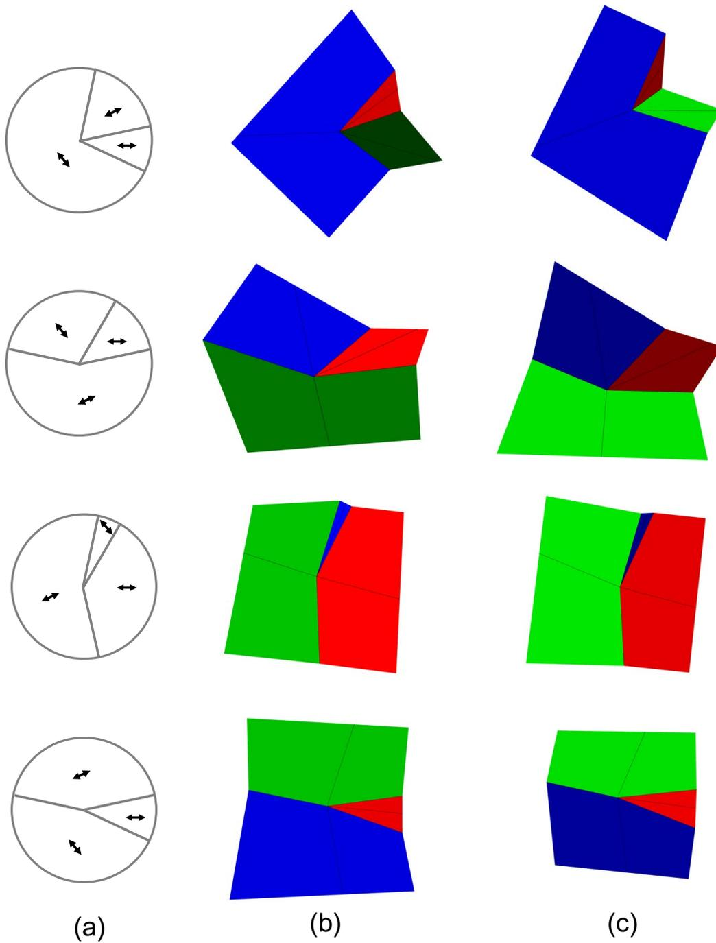
Figure 9: (a) Director design for the building block. (b),(c) The bi-stable actuations for  $r = 0.5$ .
