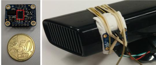
Figure 3. BNO055 board on a Kinect V1 RGB-D Camera.
