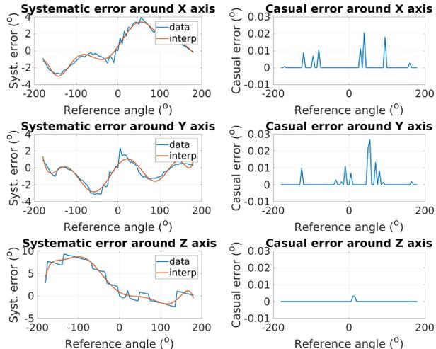
Figure 10. Uncertainty characterization of the BNO055 IMU along **X**-, **Y**- and **Z**- axes for the systematic (top) and random (bottom) errors. Note the different scales.
