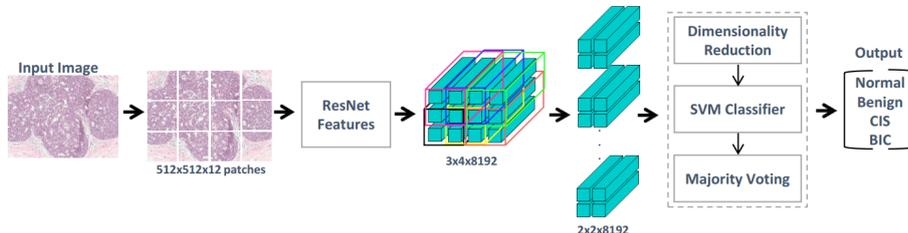
**Fig. 1.** Flow Diagram of our classification framework. Twelve non-overlapping patches are extracted from the input image. A 8192-dimensional feature vector is then obtained for each patch using a trained ResNet. The class label for the overlapping blocks ( $2 \times 2$ ) of features is obtained from the SVM model after reducing the dimensionality. The final image-based prediction is made using the majority voting approach.
