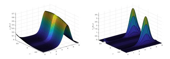
FIGURE 14. Bimodal distribution: steady state for the density  $\rho_{\infty}(\vartheta,\omega)$  (left) and  $f_{\infty}(\vartheta,\omega)$  (right) with K=2 and D=0.5.
