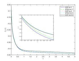
FIGURE 2. Comparison between fluxes with different  $\delta_{i+1/2}$  (3.8) and (3.18), labeled ESP2, with  $K=1,\ D=0.25$  and N=51. Solution at t=0.03 (left) and time evolution of free energies  $\mathcal{E}_{\Delta}(t)$  using different meshes.
