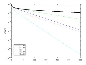
FIGURE 5. Time evolution of the log scale of the steady state  $|r(t)-r^{\infty}|$  with different values of K. Here  $r^{\infty}$  is chosen as the value of the order parameter at the final time T=1200. We observe the slowing down of the relaxation to the steady state near the critical coupling strength.
