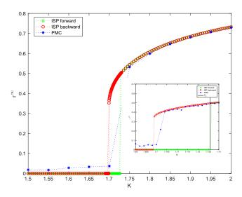
FIGURE 12. Bimodal distribution case: phase transition of the order parameter  $r^{\infty}(K)$ . ISP scheme for  $N=200,\ M=10$ . PMC method with  $5\times 10^4$  particles and 10000 averages.
