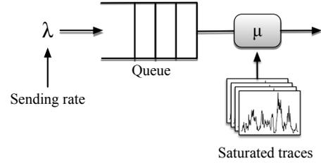
**Figure 6: The working principle of the network simulator.**
