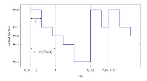
Fig. 1. Soft-TTL via time-varying fractional caching: A file i requested a times  $\tau_i(n)$  for n = 1, 2, ..., and a decreasing fraction of the file is stored in the cache for a subsequent interval of time.
