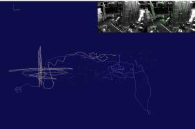
Fig. 3. Cropped screenshots of the GUI of SLAMBench2 that uses the Pangolin library [29]. On the left a point cloud extracted from ElasticFusion is shown, alongside the trajectory. The input frame and internal 3D rendering of ElasticFusion are also shown, inlaid on the right of the image. On the right a similar interface used with ORBSLAM2 and the EuRoC MAV dataset. This time the map is sparse, we can see the trajectory aligned with the ground-truth.
