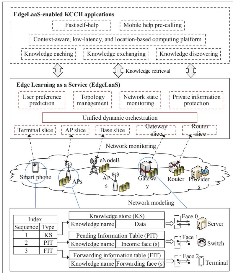
FIGURE 2. Implementation structure of the proposed KCCH.
