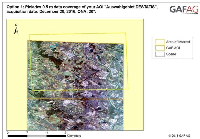
**Figure 9: The yellow rectangle shows the area of interest (AOI) for this study. The orange rectangle refers to the AOI of the satellite image provider. The bought image is the overlay area of both AOIs. The entire acquired satellite image ("scene") is shown in grey (GAF AG)**
