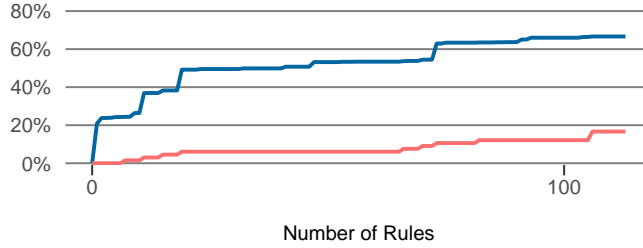
Figure 5. Influence of the number of selected rules ( Lang ). The number of rules influences the — proportion of low-fault-risk (LFR) methods and the — share of faulty methods in LFR out of all faulty methods.
