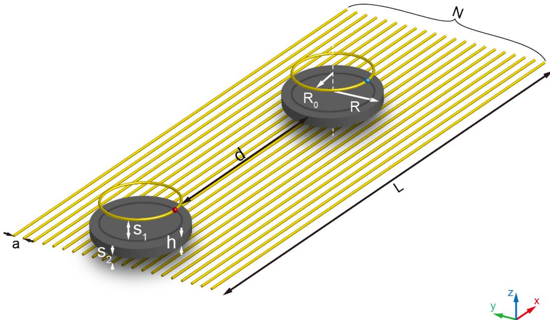
Figure 2. Geometry of proposed WPT system.
