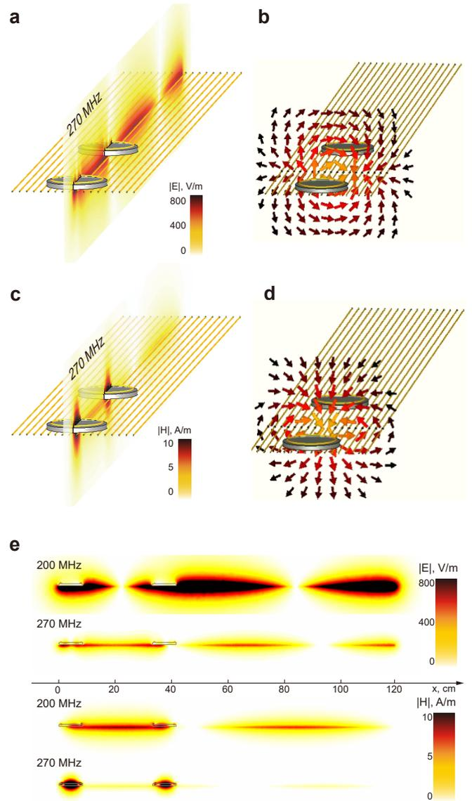
Figure 4. Simulated electric field at 270 MHz of (a) absolute value on the cross section cutting through two disk resonators and (b) vector form on the cross section half way between two resonators. Simulated magnetic field at 270 MHz of (c) absolute value and (d) vector form. (e) Comparison between electric and magnetic fields at 200 MHz and 270 MHz.
