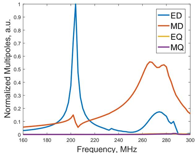
Figure 5. Multipole decomposition of the transmitting disk resonator.
