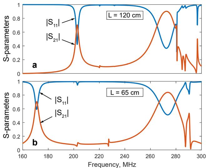
Figure 3. Comparison between the simulated S-parameter spectra of the structures with the length of metasurface (a)  $L = 120$  cm and (b)  $L = 65$  cm.
