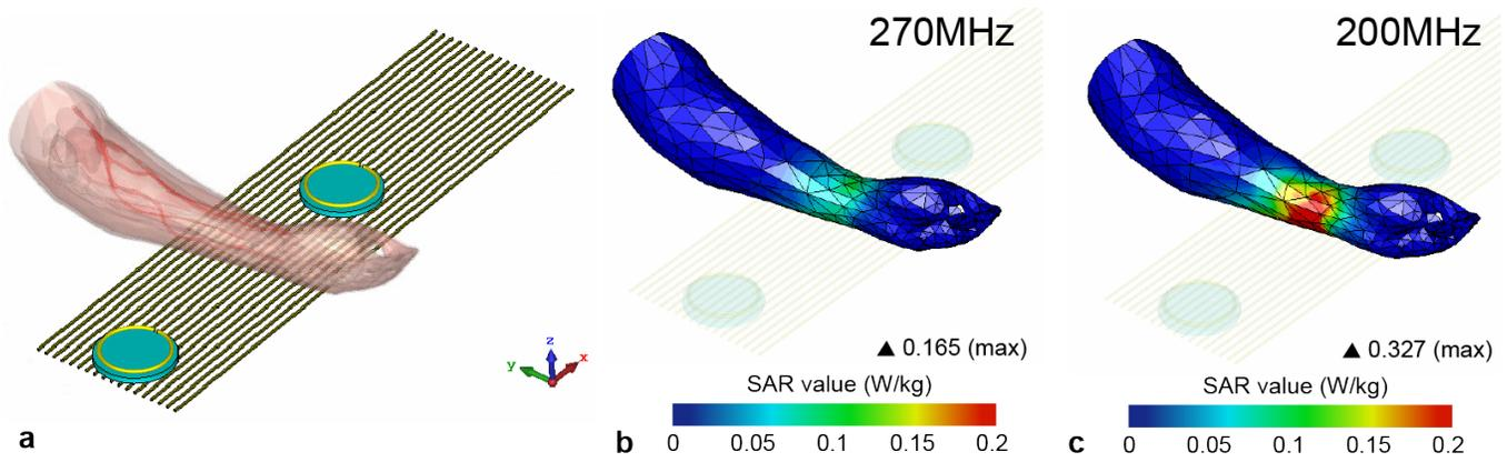
Figure 7. (a) Simulation model of the WPT system with an arm located between the resonators 2 mm above the metasurface. Simulated SAR values at the frequency of (b) ED mode and (c) MD mode.
