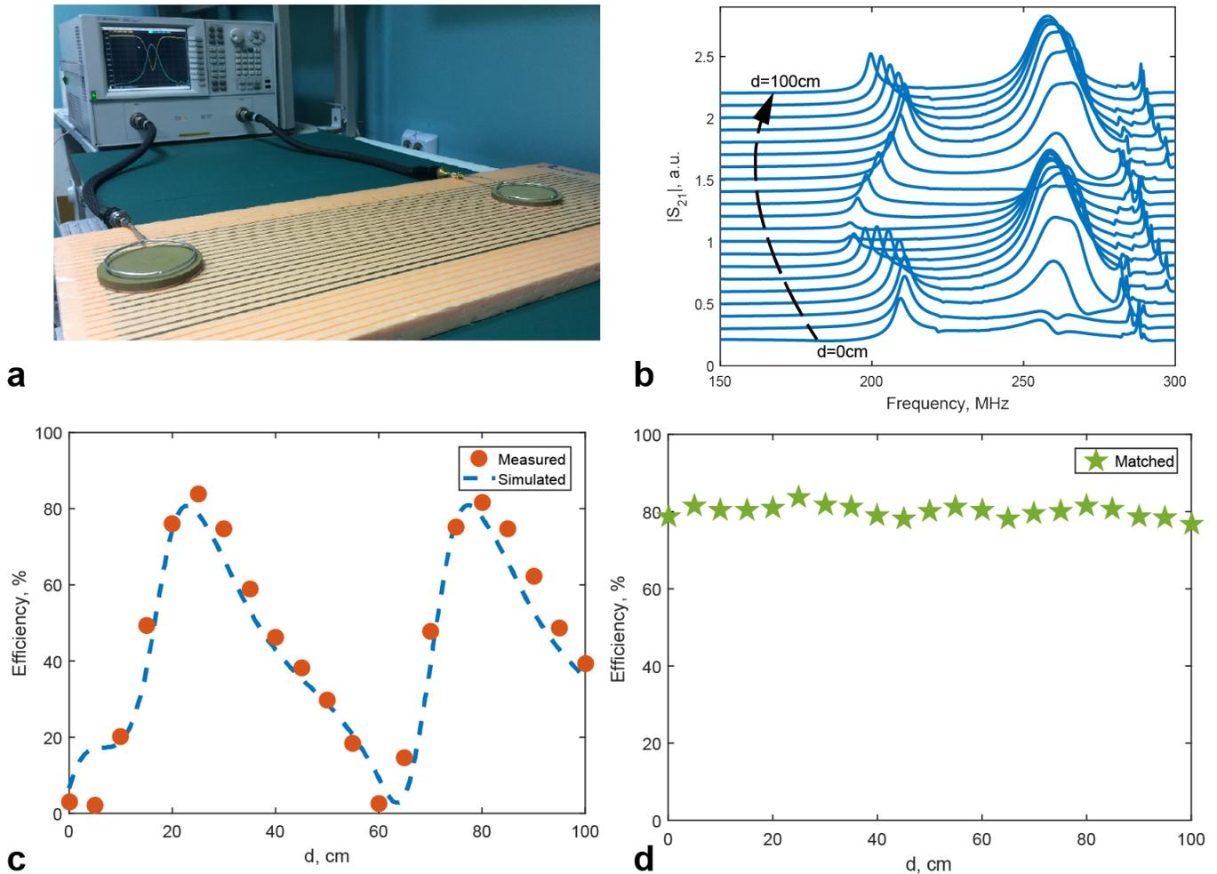
Figure 6. (a) Photo of the experiment setup. (b) Measured transmission coefficient spectra for  $d$  ranging from 0 to 100 cm. (c) Comparison between measured and simulated efficiency (d) Measured WPT efficiency when both ports are matched.
