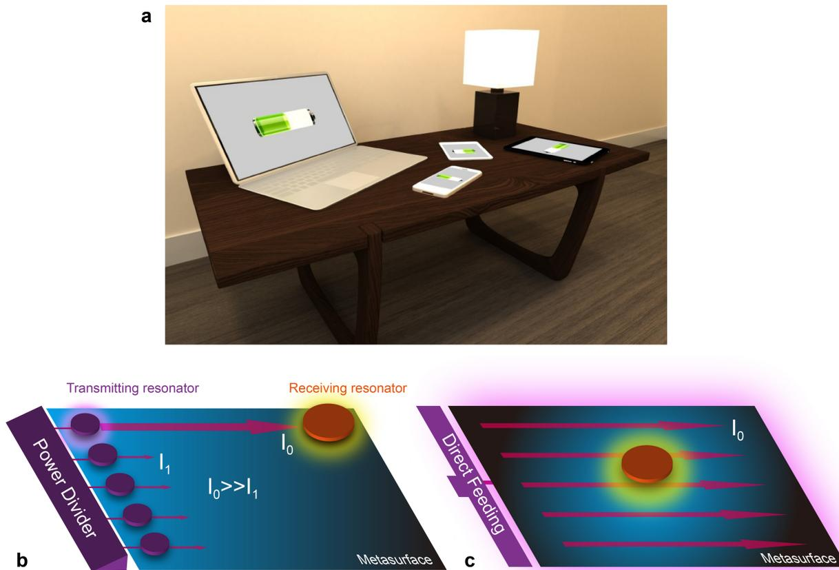
Figure 1. (a) Artist's view of multiple electronic devices being powered by a wireless charging table. (b) Metasurface as an intermediary for enhancing WPT performance. (c) Metasurface as a transmitting resonator of WPT system.
