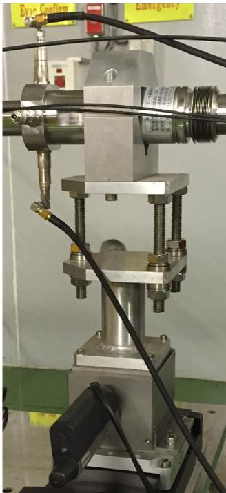
FIG. 9. Photograph of the stripline BPM P3 and its mover in the ATF beamline.
