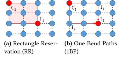
**Figure 4.** Two routing policies for swap-based architectures.
