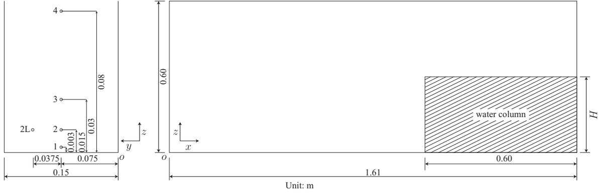
FIGURE 11. Computational model of three-dimensional dam break flow.
