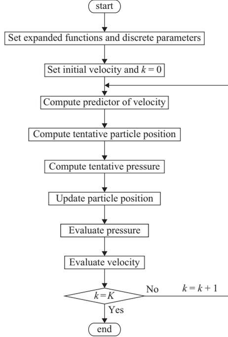
FIGURE 2. Flowchart of the explicit particle method.
