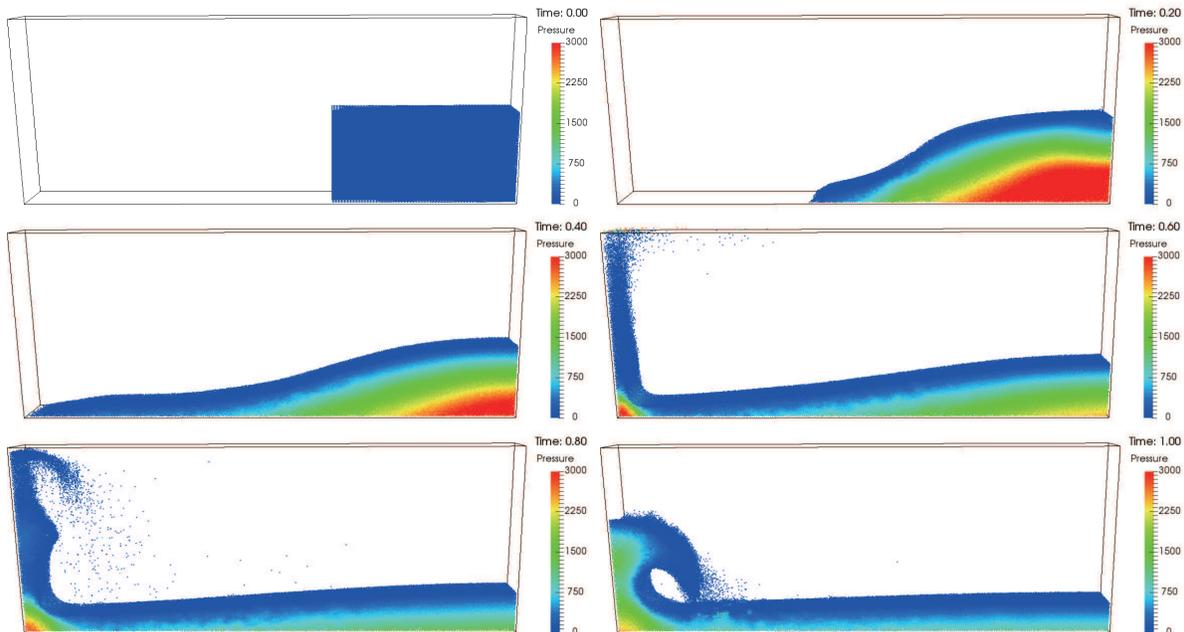
FIGURE 12. Pressure distributions for three-dimensional dam break flow ( $H_{\text{dam}} = 0.3$  m).
