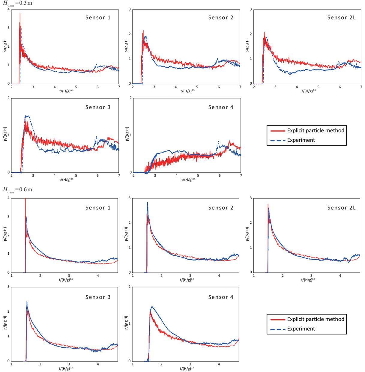
FIGURE 13. Pressure history at sensors for dam break flow.
