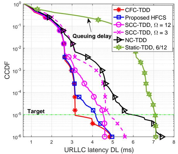
Fig. 4. URLLC outage latency in DL direction (ms).
