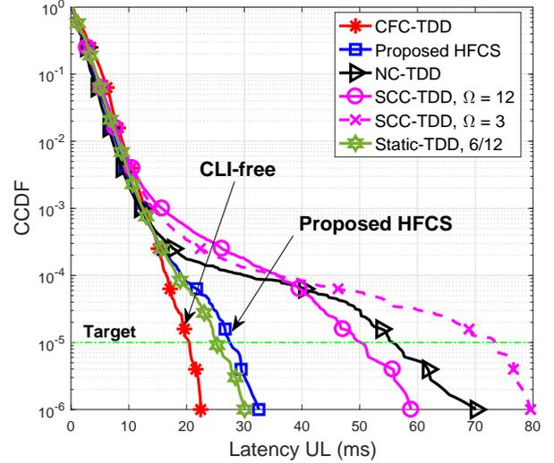
Fig. 3. URLLC outage latency in UL direction (ms).
