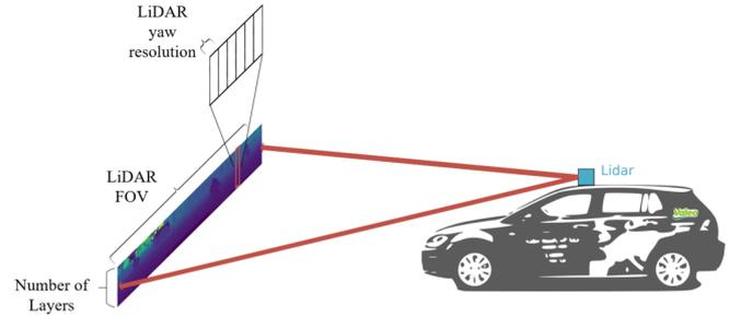
Fig. 2: Illustration of LiDAR Polar Grid Map representation.
