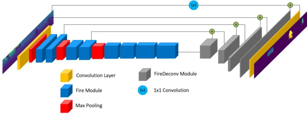
(a) LiDAR baseline architecture based on SqueezeSeg [22].
