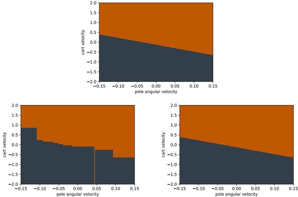
Figure 6: **Visualizing DRL (top), Viper (bottom left) and MoËT<sub>h</sub> (bottom right) policies on CartPole.** X-axis represents pole angular velocity and y-axis cart velocity, which are the most discriminatory features (topmost nodes in the Viper decision tree policy). Other features, cart position and pole angle, are set to 0 (center position with pole upright). Gray color represents points where agent takes action *left*, and orange points when agent takes action *right*.
