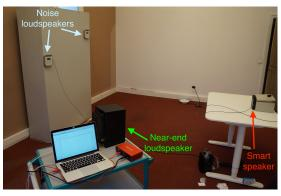
Fig. 8: Recording setup for the test set.
