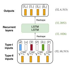
Fig. 6: Architecture of  $NN_i$  with a sequence length of 32 timesteps and F = 513 frequency bins.
