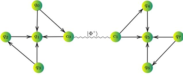
Fig. 7. Coupling map representing physical architecture of two quantum devices interconnected via the quantum teleportation paradigm. Nodes labeled with  $c_0$  and  $c_1$  denote *communication qubits*, and the dotted line indicates that they are in the entangled state  $|\Phi^+\rangle$ , i.e., they form an EPR pair. Conversely,  $q_i$  with  $i \in \{0, 1, 2, 3\}$  denote *data qubits* – i.e., qubits available for computing tasks.
