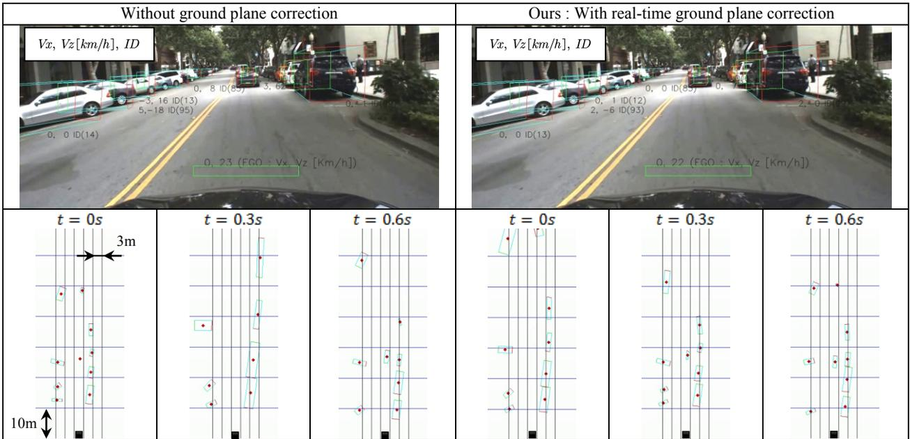
Figure 7. 3D position comparison results without ground plane correction (left) and with real-time ground plane correction (right). The vehicle positions, orientations, and bounding box size are more stable after correction.
