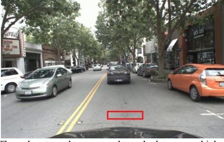
Figure 2. The red rectangular area used to calculate ego-vehicle velocity.
