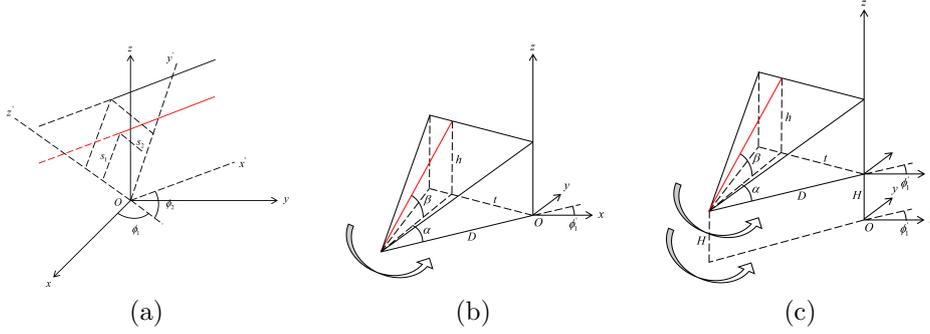
Fig. 3: (a) 3D parallel beam; (b) Circular cone beam; (c) Helical cone beam
