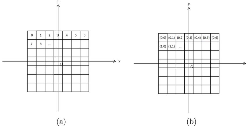
Fig. 2: (a) Pixel index in 1D form; (b) Pixel index in 2D form
