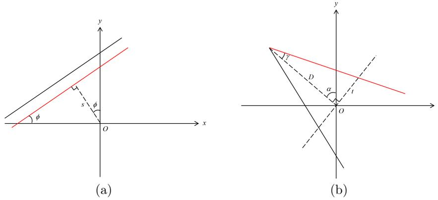
Fig. 1: (a) 2D parallel beam; (b) Fan beam
