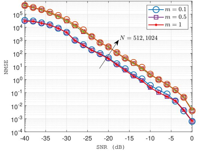
Fig. 6. GAT can perform accurate channel estimation under varying solar scintillation effects, which can be grouped into weak ( $m < 0.3$ ), transition zone ( $0.3 \leq m < 1$ ), and strong scintillation ( $m = 1$ ). The circular, square and dot markers denote misalignment index  $m = 0.1, 0.5$ , and 1, respectively.
