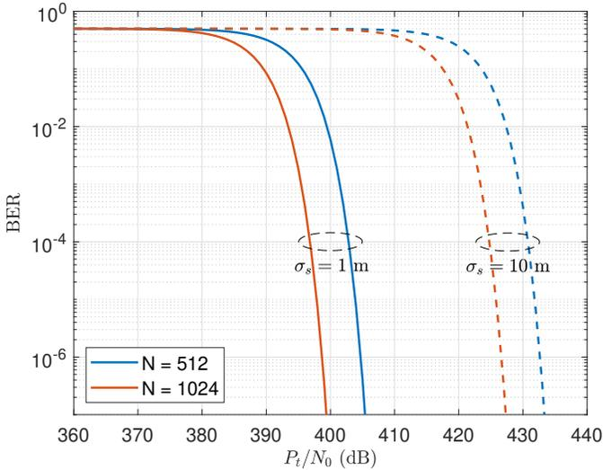
Fig. 5. BER versus  $P_t/N_0$  under the misalignment fading, which can seriously decrease the communication performance in terms of error probability, for BPSK signaling. The radius of equivalent beamwidth is chosen as 10 m and  $\sigma_s$  denotes the misalignment jitter.
