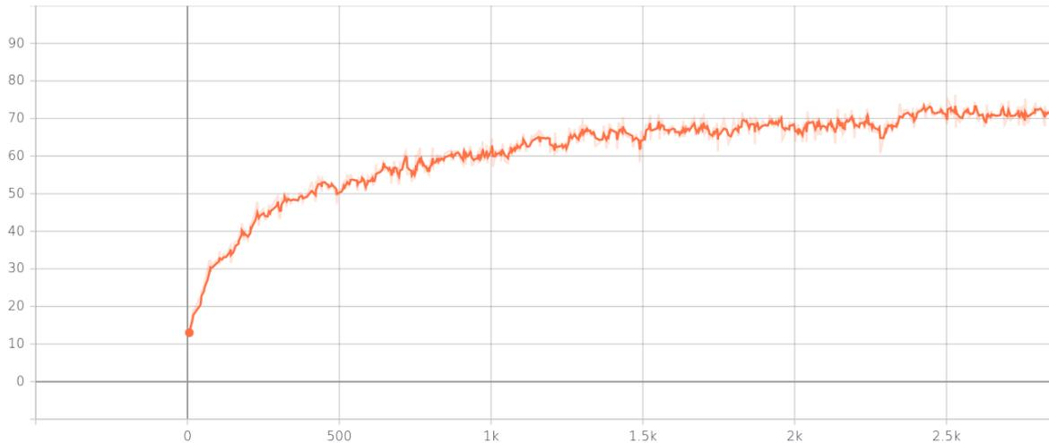
Figure 7.2: Training curve for a successful in-hand manipulation task. Shown on the horizontal axis is the number of policy updates. Each update consists of 96 episodes of 64 steps each.
