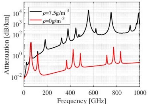
Fig. 14. The specific attenuation due to atmospheric gases.
