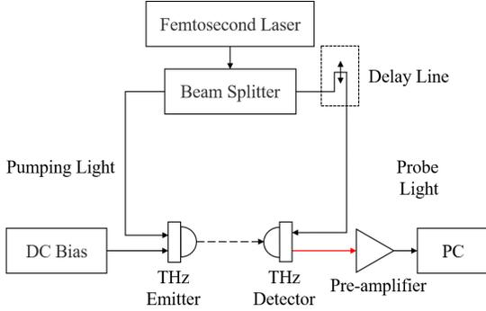
Fig. 5. The architecture of a pulse-based measurement system.
