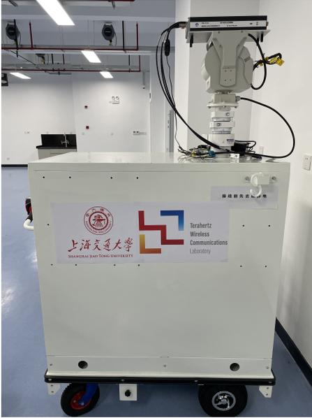
Fig. 3. The 260-400 GHz VNA-based channel measurement system.
