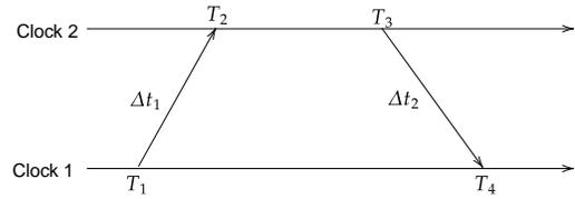
FIGURE 4. Operating principle of the TWTT clock synchronization [28]
