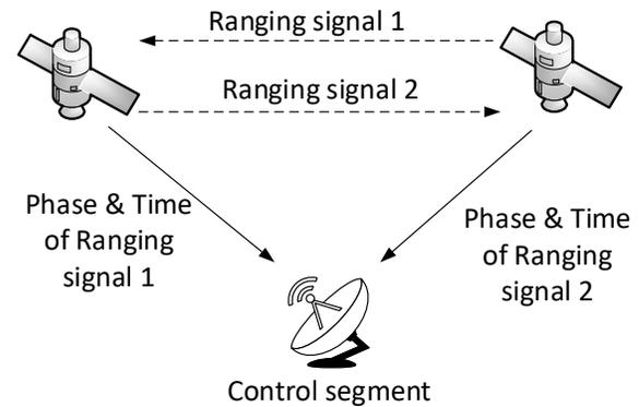
FIGURE 9. Basic principle of RF carrier-ranging by DOWR.
