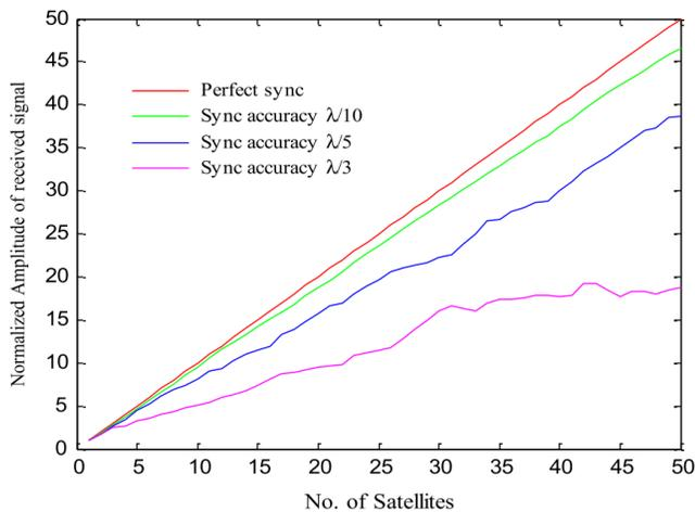
**FIGURE 10.** Normalized amplitude of the received signal vs. the number of satellites for different values of phase synchronization accuracy [8]
