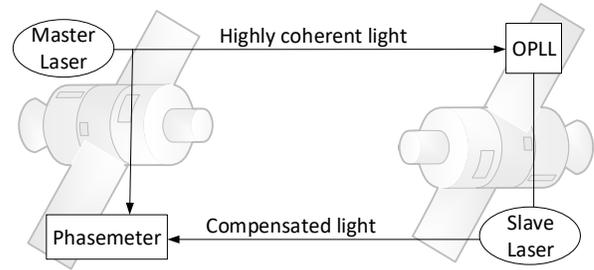
FIGURE 8. Basic principle of optical inter-satellite ranging measurement
