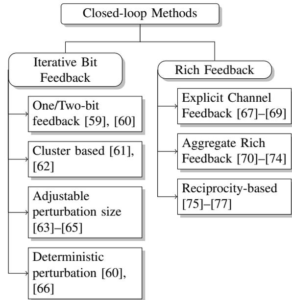
FIGURE 5. Classification of the Closed-loop synchronization methods
