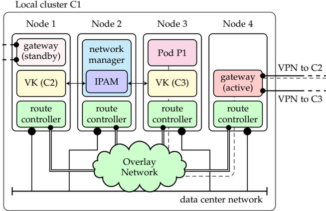
Fig. 5. Main *liqo* components of the network fabric subsystem, including the interconnection between clusters. The dashed line shows the path followed by traffic originating from a pod P1 and directed to one hosted on cluster C2, flowing through the overlay network to reach the gateway pod and eventually entering the VPN tunnel.
