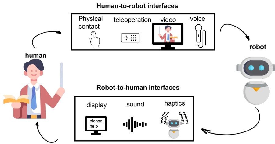
Figure 9.1: Human-to-robot interfaces and robot-to-human interfaces commonly employed in III.
