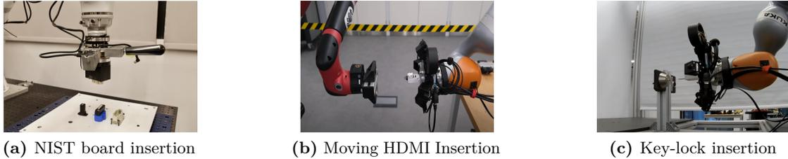
**Figure 11.14:** Robot in Assembly Tasks. Source: (Luo *et al.*, 2021).
