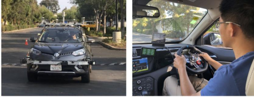
**Figure 11.7:** Test vehicle (left) and expert driver interface (right). Source: (Kelly *et al.*, 2019).
