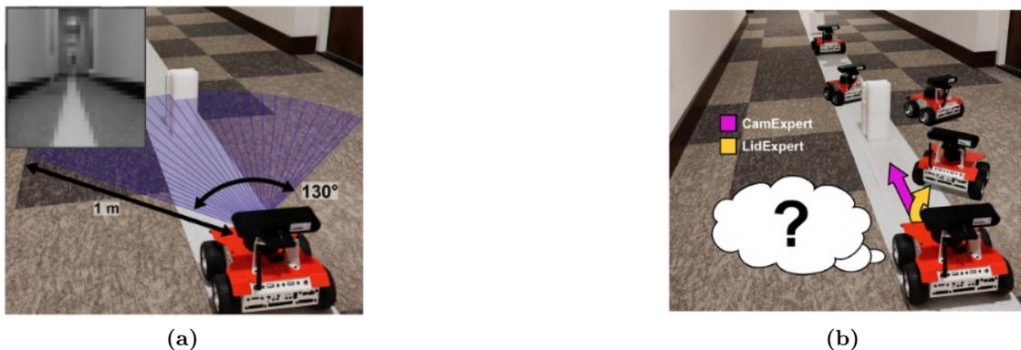
**Figure 11.8:** Learning navigation behavior for an autonomous mobile robot. The figure shows conflicting decisions based on two different sensory feedback. In conflicting situations, an expert is queried to take control and the correct action of a sensor-fused policy. Source: (Bootsma *et al.*, 2021).
