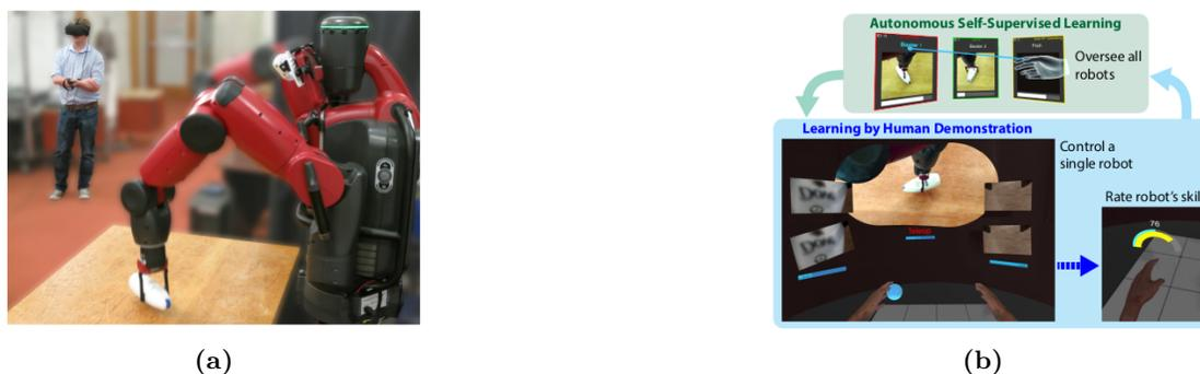
**Figure 11.2:** Figure (a) shows the setup where a person supervises a robot for a grasping task. (b) shows the virtual reality interface where the user remotely gives grasping demonstrations. Source: (DelPreto *et al.*, 2020).
