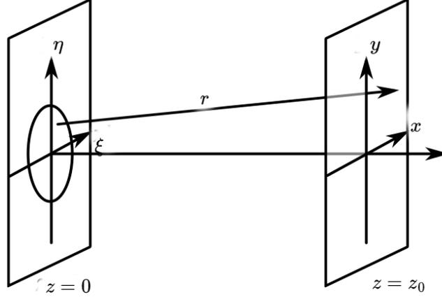
**Fig. 7.** A schematic diffraction imaging system with parallel aperture and imaging planes (plot adapted from [https://commons.wikimedia.org/wiki/File:Diffraction\\_geometry.svg](https://commons.wikimedia.org/wiki/File:Diffraction_geometry.svg) under the Creative Commons Attribution-Share Alike 3.0 Unported license.)
