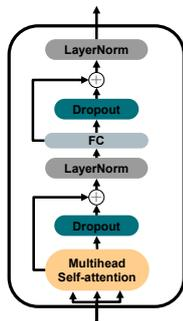
Figure 2: Transformer Encoder.
