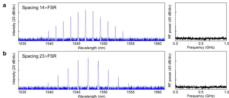
**Fig. S4 | Soliton crystal states generated in 10.1 GHz FFPR.** Left panels: spectra of soliton crystal states with comb spacings of 140 GHz and 230 GHz, respectively. Right
