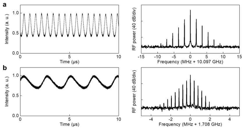
**Fig. S5 | Breather soliton states.** Left panels: time domain signals. Right panels: RF signals. **a**, 10.1 GHz microcomb. **b**, 1.7 GHz microcomb.
