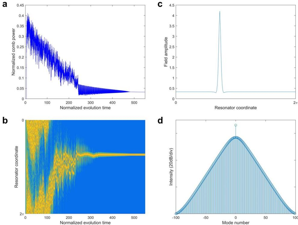
**Fig. S1 | Numerical simulations of self-injection locking soliton microcomb**
