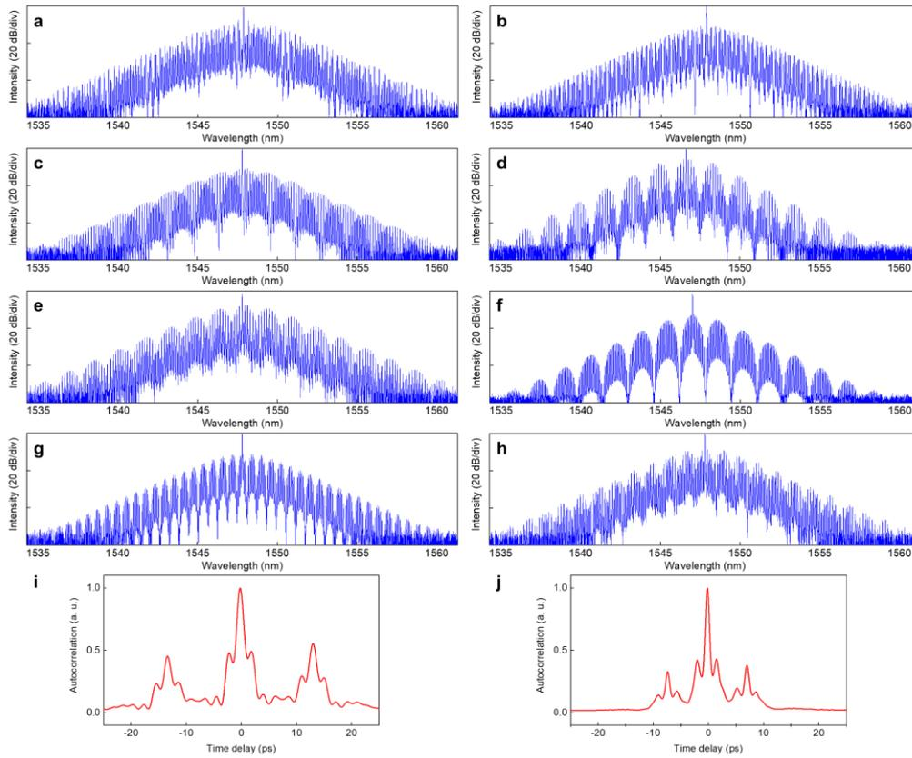
**Fig. S2 | Multiple soliton states generated in 10.1 GHz FFPR. a-h**, spectra of multiple soliton states. **i, j**, autocorrelation traces of multiple soliton states in **g** and **h**, respectively.
