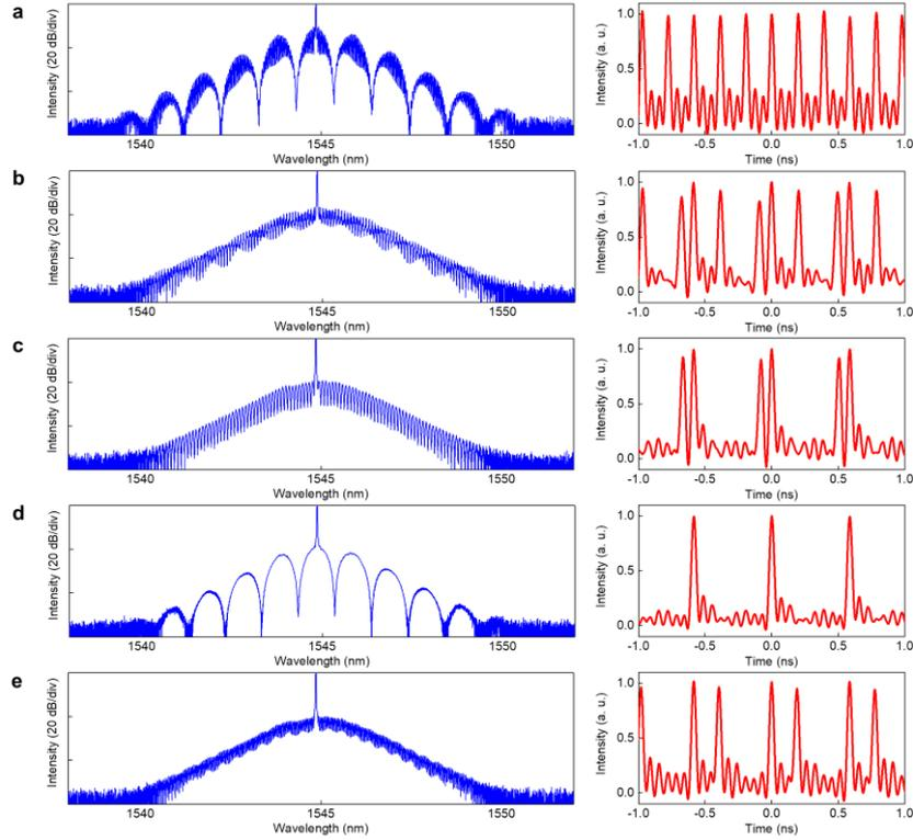
**Fig. S3 | Multiple soliton states generated in 1.7 GHz FFPR.** Left panels: spectra of multiple soliton states. Right panels: pulse trains measured by a fast-speed oscilloscope.
