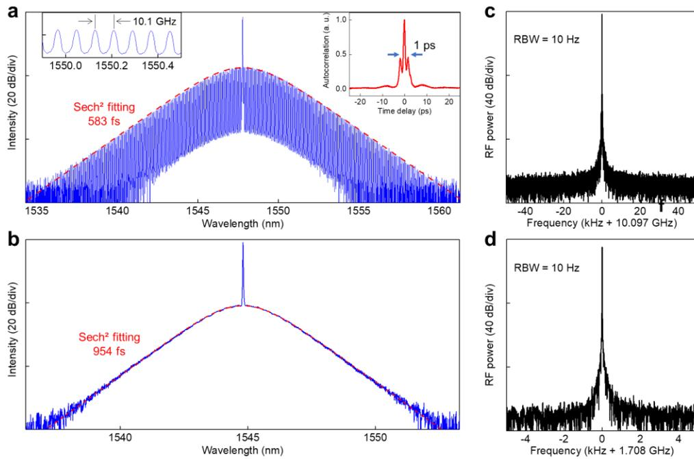
**Fig. 3 | Single soliton generation.** **a, b**, Optical spectra of single soliton states at 10.1 GHz and 1.7 GHz, respectively. Left inset of **a**: zoom-in spectrum of 10.1 GHz comb lines (OSA resolution is 0.02 nm). Right inset of **a**: autocorrelation trace of 10.1 GHz single soliton pulse. **c, d**, RF beatnotes of single soliton states at 10.1 GHz and 1.7 GHz, respectively. RBW, resolution bandwidth.
