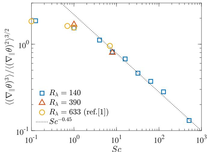
FIG. 1. Skewness of  $\nabla_{\parallel}\theta$  as a function of  $Sc$ , for various  $R_{\lambda}$ . The data for  $R_{\lambda} = 390$  and  $633$  are respectively adjusted by factors 1.2 and 0.9 to account for a very weak  $R_{\lambda}$  dependence, but do not have any bearing on trends with  $Sc$ .
