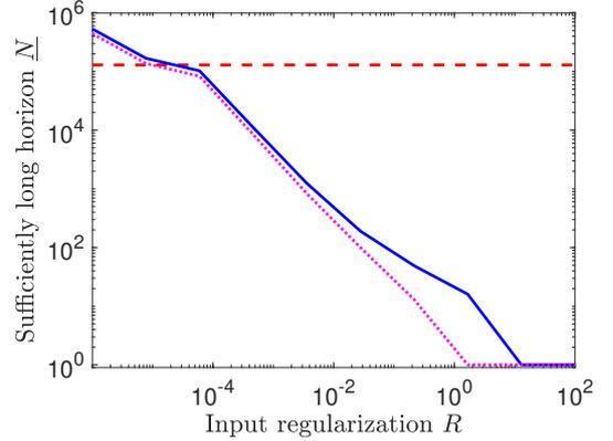
Figure 5: Chain of mass–spring–dampers, adapted from Köhler et al. (2023). Sufficient horizon  $\underline{N}$  for stability for varying  $R$  based on Theorem 11 in blue, solid. Bound  $\underline{N}$  utilizing an additional approximate terminal cost (Sec. 6.3.2) using a finite-horizon roll-out with  $M = 10$  shown in magenta, dotted. Theoretical bounds  $\underline{N}$  using Theorem 10 shown in red, dashed.
