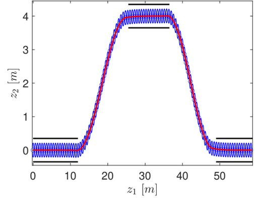
Figure 1: Evasion manoeuvre of a car with reference trajectory  $r$  (red), (projected) terminal sets (blue ellipses) and state constraints (black), adapted from Köhler et al. (2020a). The terminal ingredients are optimized offline before knowing the exact reference trajectory  $r$  (cf. Sec. 3.4).
