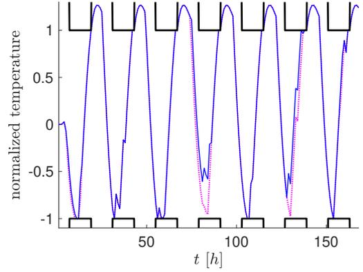
Figure 4: Temperature control in a building, adapted from Köhler et al. (2020c). Closed-loop state  $x$  (blue, solid) resulting from periodic economic MPC (Thm. 9) with time-varying ambient temperature and price signal, which also changes unpredictably during online operation. Time-varying state constraints (black, solid). Optimal trajectory computed in hindsight with known price signal  $y_e$  shown in magenta, dashed.
