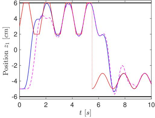
Figure 3: Periodic tracking with a ball-and-plate system, adapted from Köhler et al. (2020b). Closed-loop state  $x$  (blue, solid) resulting from periodic tracking MPC (Sec. 4.3.1) with a time-varying target signal  $y_d$  (red) and state constraints  $\mathbb{X}$  (black). Closed-loop state resulting from partially decoupled tracking and planning (Sec. 4.4) with  $M = 2$  shown dashed in magenta.
