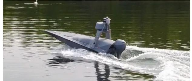
Fig. 1. Piraya autonomous unmanned surface vehicle. Courtesy of <https://portal.waraps.org/>
