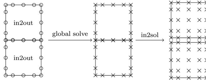
Figure 2: Solution strategy of both element learning and the standard HDG method. To create a global solver, the local solvers (in2out operators, from Figure 1) from neighboring elements are coupled together. In this schematic diagram, we use ‘o’ for undetermined DOFs and ‘x’ for determined DOFs (solved solution).
