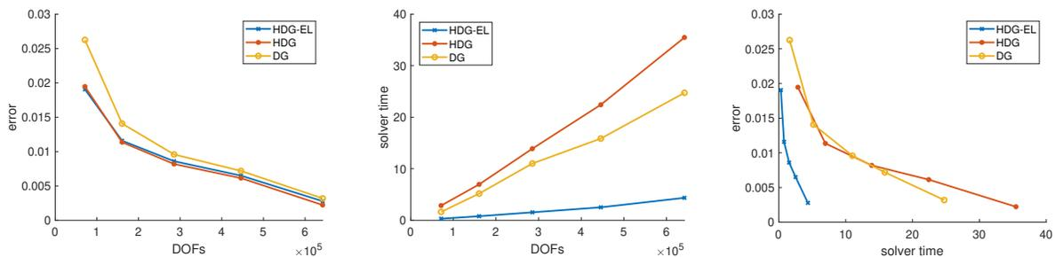
Figure 14: Comparison of the different methods in terms of cost and accuracy, for the I3RC test case. Left: DOFs vs relative  $L^2$  error. Middle: DOFs vs solver time. Right: solver time vs relative  $L^2$  error. The solver time for HDG and HDG-EL is the summation of the local solver and the global solver time. For an error level of approximately  $2 \times 10^{-3}$ , in the right panel, the HDG-EL method is 5 to 10 times faster than the DG and HDG methods.
