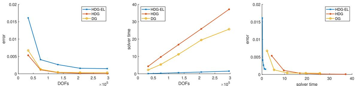
Figure 10: Comparison of the different methods in terms of cost and accuracy, for test case 1. Left: DOFs vs relative  $L^2$  error. Middle: DOFs vs solver time. Right: solver time vs relative  $L^2$  error. The solver time for HDG and HDG-EL is the summation of the local solver and the global solver time. For an error level of approximately  $2 \times 10^{-3}$ , in the right panel, the HDG-EL method is around 5 to 10 times faster than the DG and HDG methods.
