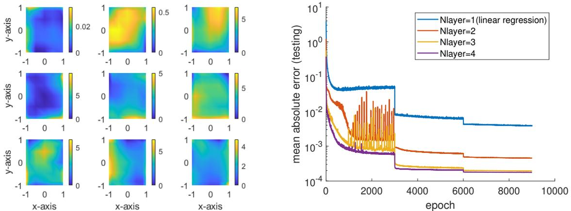
Figure 5: Training the neural network. Left: 9 samples of the scattering coefficient  $\sigma_s$  generated from the Algorithm 2. Right: testing error for the networks with different number of layers. The testing error is lowest (and similar) for 3 or 4 layers. The neural network is able to learn the nonlinear operator from (16) with an error that is nearly as small as  $10^{-4}$ .
