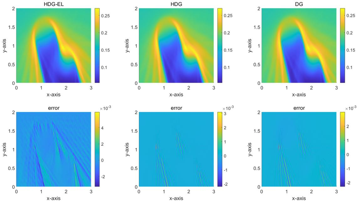
Figure 9: Numerical solution and error landscape for the test case 2 (right figure of Figure 7), with steeper gradient at cloud boundary. Top row: numerical solution (mean intensity) obtained by HDG-EL, HDG, and DG methods in the refinement level  $l = 4$ . Bottom row: error landscape of the corresponding methods. All methods achieve a similar error level of  $10^{-3}$ .
