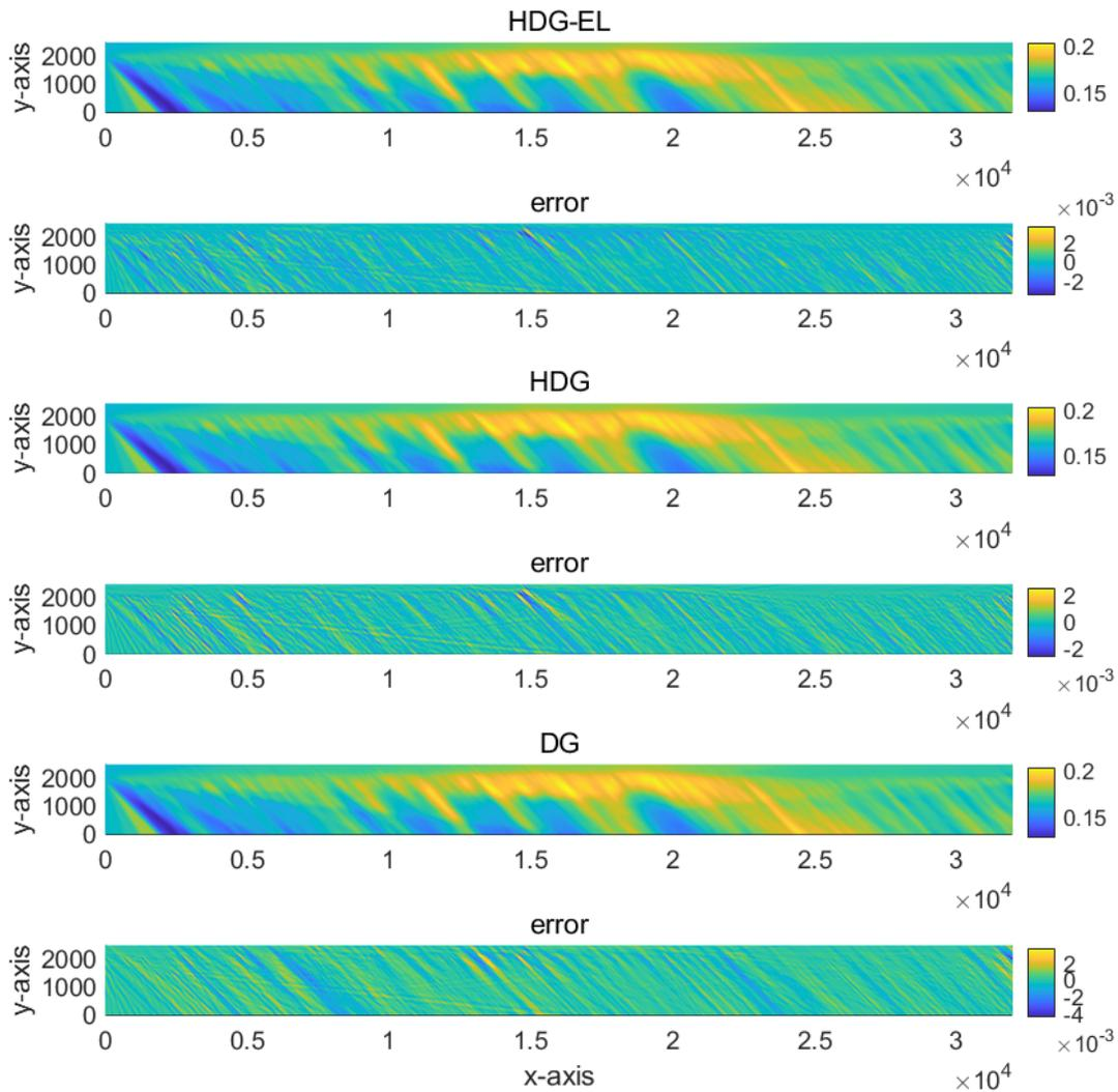
Figure 13: Numerical solution and error landscape for I3RC test case (see Figure 12). Odd row: numerical solution (mean intensity) obtained by HDG-EL, HDG, and DG methods in the refinement level  $l = 4$ . Even row: error landscape of the corresponding methods. All methods achieve a similar error level of approximately  $2 \times 10^{-3}$ .
