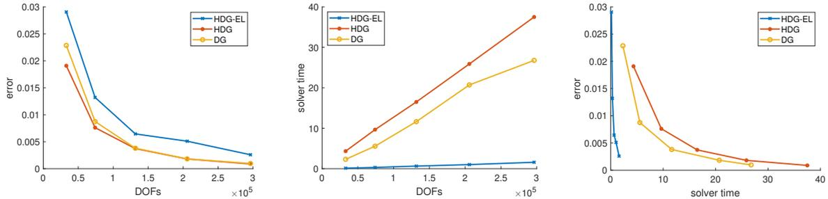
Figure 11: Comparison of the different methods in terms of cost and accuracy, for test case 2. Left: DOFs vs relative  $L^2$  error. Middle: DOFs vs solver time. Right: solver time vs relative  $L^2$  error. The solver time for HDG and HDG-EL is the summation of the local solver and the global solver time. For an error level of approximately  $2 \times 10^{-3}$ , in the right panel, the HDG-EL method is around 10 times faster than the HDG and DG methods.
