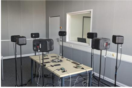
Figure 1: Recording setup of *LibriWASN*<sup>200</sup>: Eight loudspeakers surrounding a table with multiple recording devices.
