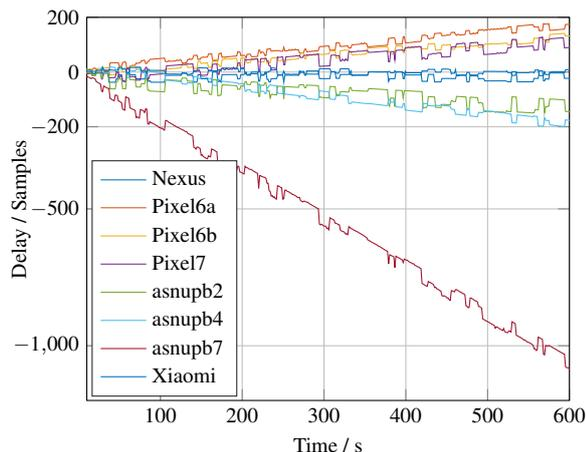
Figure 4: Estimated delay between soundcard and first channel of each device (*LibriWASN*<sup>200</sup>, OV40, Ses. 9).
