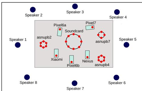
Figure 2: *LibriWASN*<sup>200</sup> recording and playback devices: Eight loudspeakers surrounding a table with 5 smartphones, one 8-channel microphone array (soundcard) and three Raspberry Pi devices. Red dots indicate microphones on devices.
