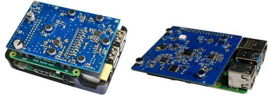
Figure 3: Raspberry Pis with mounted soundcards. Left: AudioInjector Octo with 6 channel microphone analog frontend (*asnupb2* & *asnupb4*). Right: FPGA-based 4 channel soundcard (*asnupb7*).
