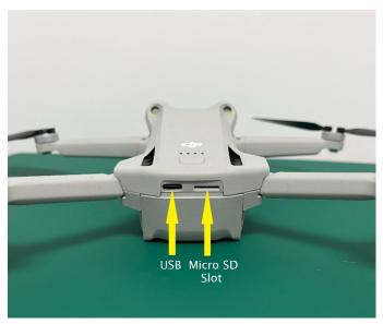
Fig. 6. A view of the USB port and Micro-SD card slot on the Mini 3 Pro.
