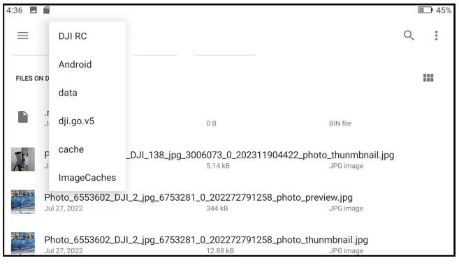
Fig. 17. Thumbnail images discovered on the RC's internal memory via the RC files utility.
